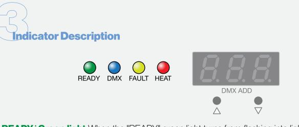
**READY: Green light** When the "READY" green light turns from flashing into light on, it indicates that the machine is ready to work.
