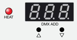
$\triangle$ : Means increasing DMX address code; long press helps increase fast.  $\nabla$ : Means decreasing DMX address code; long press helps decrease fast.
